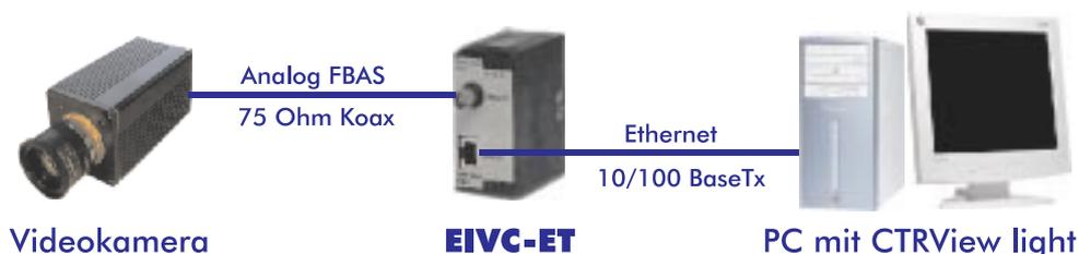
This is the minimal application for the videoconverter. The IVC-ET captures the pictures from the camera via composite video, transports them via Ethernet with 10/100BaseTX to a PC with the CTRLView light software.
